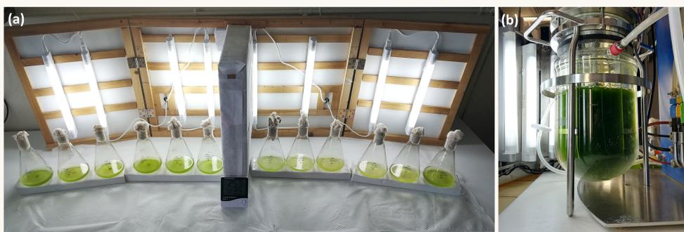
**Figure 2.** Bioreactors used in this investigation: (a) Erlenmeyer flasks 0.5-L ( $V_w = 0.1$  L) and (b) STR 3.7 L ( $V_w = 2.0$  L).  $V_w$ : working volume.
